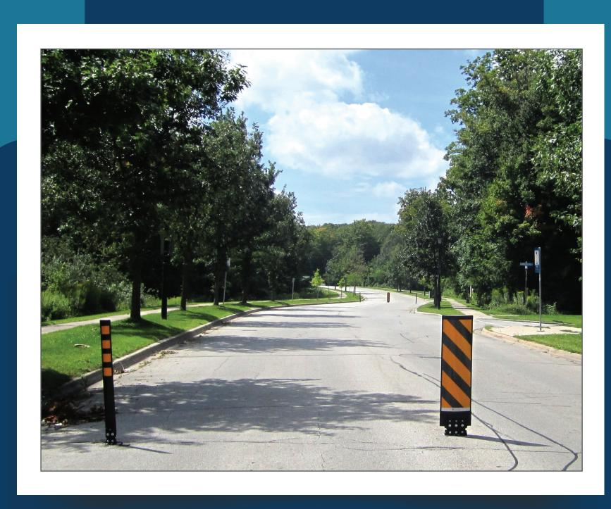
Flexible delineator posts that reduce roadway width.
