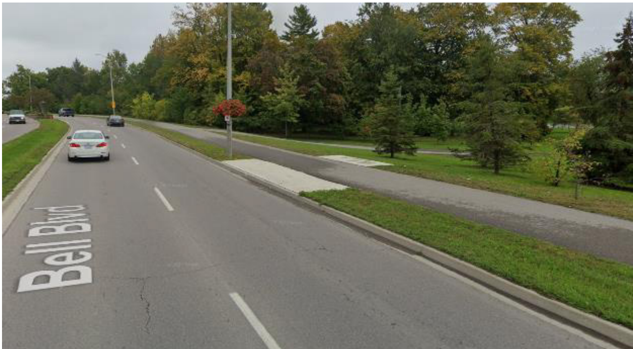
Figure 66: Belleville Transit Bus Stop on Bell Boulevard at Riverside Park. This is a far-side stop with a pad connected with a multi-use trail.
