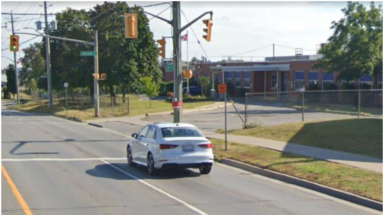
Figure 62: Belleville Transit Bus Stop on Sidney Street at Graham Street. This is a near-side stop on an arterial road with no pad or shelter.
