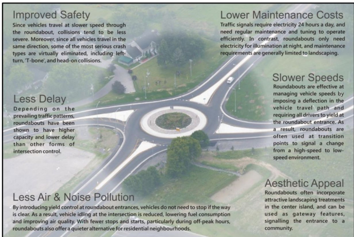
Figure 6: Benefits of Roundabouts, as illustrated in the City of Belleville Transportation Master Plan (2014).
